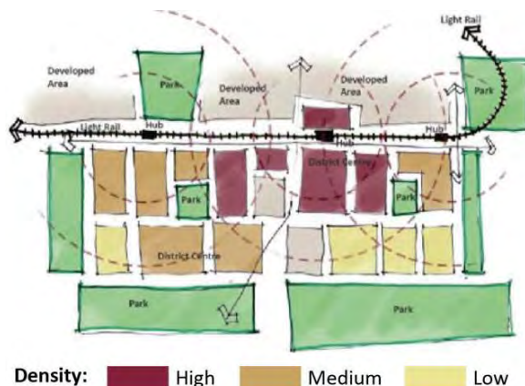
Figure 14.11 - Plan of a Transit-Oriented Development (Source: 2022-2042 Transport Strategy for the GDA)
